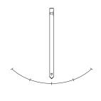
RACK should swing freely on the mounting disc so that you may level it vertically.
