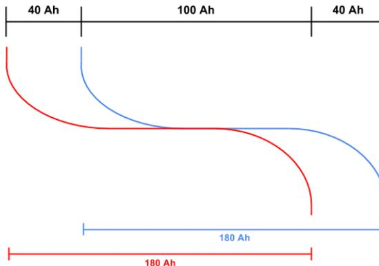
3. A correction drift may occur if the capacity of the cells has changed due to cold temperatures. Some cells (notably iron-phosphate cells) have a restricted range in the cold which can be as little as 50% of the normal capacity. Newer versions of the Orion BMS firmware have compensation for this effect to avoid SOC drift, but if this is not setup, an SOC correction will occur due to the reduced capacity in the same way it does for the above issues.
