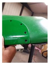
4. With the hardware provided install the self tapping screws in each of the predrilled holes on the wear panel.
