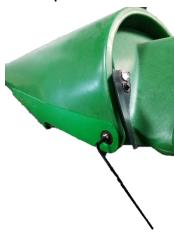
3. Using a 3/16 drill bit drill out into the snout through the predrilled part as shown and insert the hardware provided do not over tighten as this could affect the strength of the wear part.
