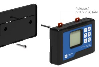
Determine where to locate the main controller. The controller comes with a simple to use DIN type bracket. Pull the 4 tabs outward to release the bracket from the unit, mount the bracket to a wall or surface, place the unit back on the bracket and press the 4 tabs back in to lock the unit in place.
