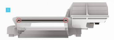
The reflector can be taken out by carefully unlatching the top of the reflector from the holding pins in the reflector cover (image 2 and 3).
