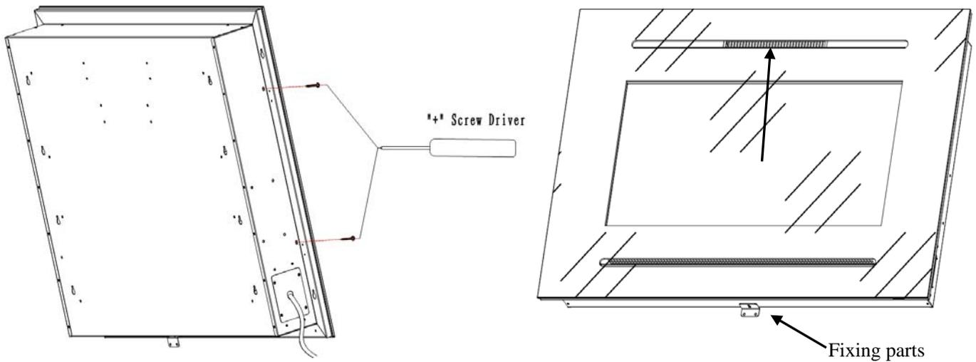
2. Doing the test before installing, then insert the firebox into the hole.
