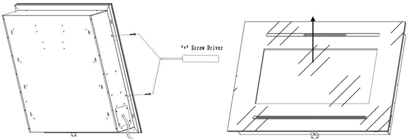
2. Doing the test before installing, then hang the back hole of the fireplace to the installed hanging nail in advance. As picture.
