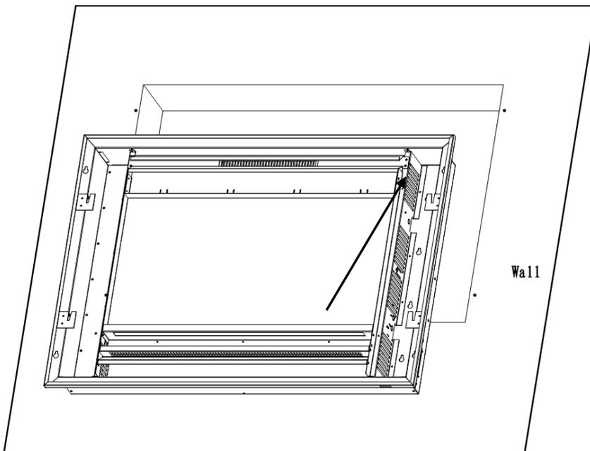
3. Use the self-tapping ST5x37 to thread to the bulged screw tube with the "+" screw driver, Ensured that the fireplace fixed on the wall and it can't move.
