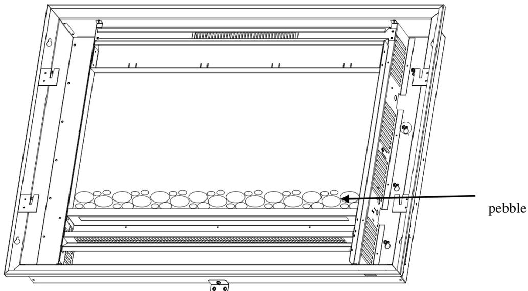
5. Install the glass according to the steps of the removing.
