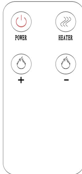
**Power** Press the power button on the remote to turn the flame on and off.
