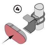
4. Insert the light into the bracket by pushing down as illustrated.
