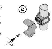
2. Locate the grey rubber pad from the top bracket and mount the bracket on top of the base part. Insert the screw with the small O-ring and tighten it using the included Allen key.
