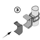
3. Insert the grey rubber pad into the top bracket.
