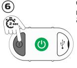
**6.** Turn on the light by pressing the button down for 2 seconds.
