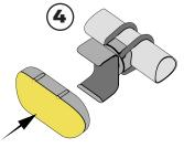
**4.** Insert the light into the bracket by pushing down as illustrated.
