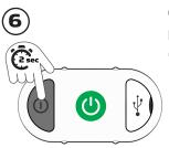
**6.** Turn on the light by pressing the button down for 2 seconds.
