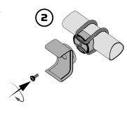
2. Locate the grey rubber pad from the top bracket and mount the bracket on top of the base part. Insert the screw with the small O-ring and tighten it using the included Allen key.
