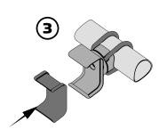
3. Insert the grey rubber pad into the top bracket.
