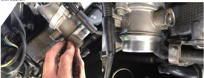
6) Apply Loctite to leading edge of ASV fitting completely around as pictured (the tube may require some persuasion to get Loctite out but it contains enough for the application).
