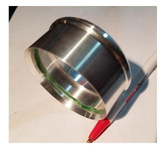
7) Slide ASV fitting onto ASV while twisting, this will insure good coverage/bonding. Be careful to keep the fitting straight. Slide fitting on until the angled section fully seats as shown.
