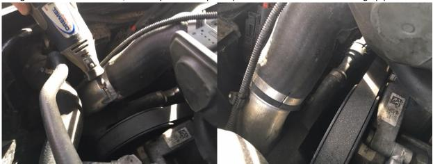
3) Unclip ASV electrical connector (circled). Pull quick-release clip outwards from hose and slide factory connector off of ASV. Push clip back in to pull off completely. Remove elbow from cold-side pipe as well.
