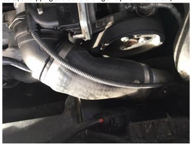
2) Using Dremel or cutoff wheel, carefully cut factory clamp that holds boot cold side charge pipe
