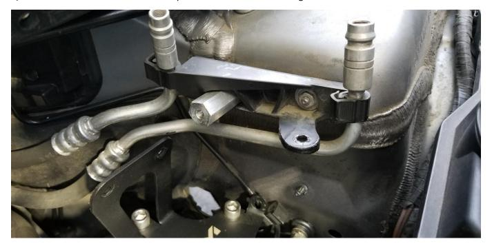
4) Put filter bracket assembly in place to check cowl hole locations. If needed they can be enlarged to aid with fitment. Do not mount assembly at this time.
