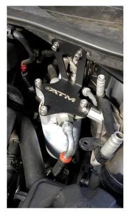
9)Install filter if not already done so. Smaller rubber washer goes on housing threads first. Use lubricant on rubber o-ring surface
