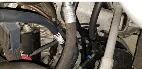
8)After confirming safe routing of all hoses, mount filter assembly and tighten. \*\*Insure there is adequate clearance between all hoses, especially in relation to steering shaft\*\* If needed loosen outlet elbow at filter housing and reposition.
