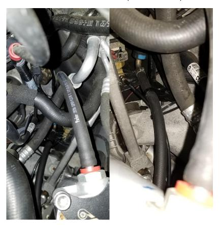
6)Disconnect factory quick release fittings and connect respective ends to filter hoses.
