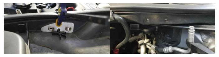
3) Remove nut on AC line bracket and replace with hex standoff and tighten.
