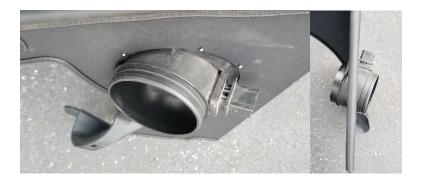
4) Place air filter on MAF and locate intake shield in place. Insert front ear of shield into radiator support and route single connector and main harness into cutout as shown. While pulling inlet boot out of the way, push intake in place over lower stud.
