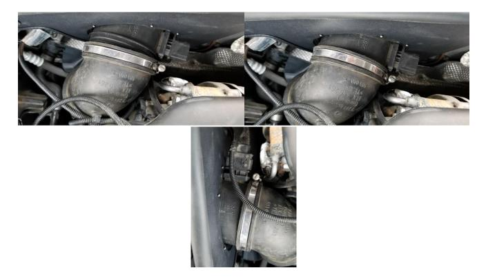
6) Insert hold-down into slot as shown. Tighten down using included washer w/factory bolt. Tighten supplied nut/washer onto bottom stud
