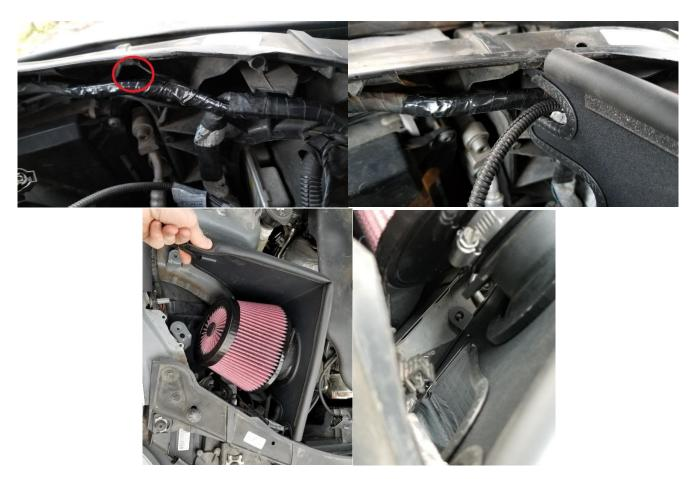
5) Plug in MAF sensor connector, listening for audible "click". Connect inlet hose to MAF and tighten.
