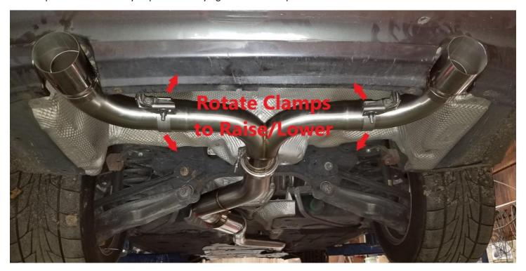
14)Install tips with clamps and adjust as necessary. Tighten.
