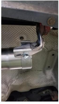
13)Tailpipe elbows can now be adjusted in and out as well as up and down as needed. If overall height of the Y-pipe needs to be adjusted band clamps can be rotated to raise/lower system. The tailpipe elbows should be centered with the bumper cutouts as closely as possible. Fully tighten band clamps.
