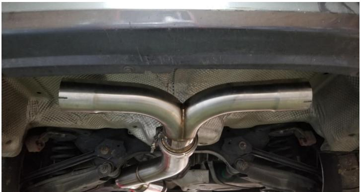
11)Confirm rear midpipe placement is correct (centering between diff and suspension arm will be adjusted later), level rear Y-pipe as close as possible and tighten V-band clamp. Midpipe hanger can also be adjusted if necessary to provide proper clearance.
