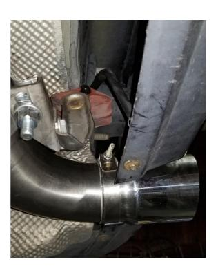
15)Check entire system for clearance and adjust if needed. Ensure all clamps/brackets are tight.
