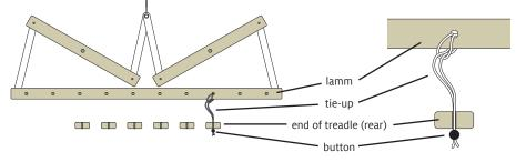
FIGURE 6: INSTALLING TIE-UPS
