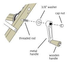
FIGURE 3: INSTALLING THE WARP BEAM CRANK HANDLE
