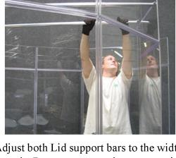
13. Adjust both Lid support bars to the width of the font panels. Rest one support bar on top with the J-hooks at least 4-inches from the edge of the end panels. Place the other bar about a foot in front of the first bar. Do not extend the bar beyond the red limit mark.
