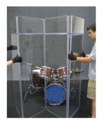
8. With one person on each side, unfold the system and wrap it around the kit.
