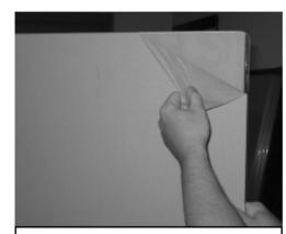
**3.** Peel masking off panels. Wear gloves when handling acrylic to avoid fingerprints.
