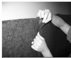
7. Move the S2466x2 baffles into position behind kit. Use the Velcro flaps on outside top and bottom sides of S2466x2 to attach the units together. Ends of baffles should overlap inside of shields or butt up against them.
