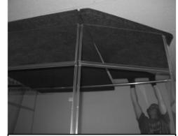
**12.** Lay ST2466 trapezoids on either side of center lid section. Leave at least an inch over-hang in front. Make sure AX height extenders stay upright and perpendicular to floor.
