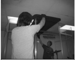
11. Lay rectangular S2466 on top center of IsoPac with at least a one inch over-hang in front and resting on support bar in back.
