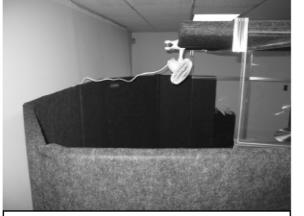
17. Leave a small opening in upper back of IsoPac to allow for some air exchange. If necessary, overlap \$2466x2 and end shields to decrease opening.
