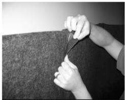
9. Move the S2444x2 baffles into position behind kit. Use the Velcro flaps on outside top and bottom sides of S2444x2 to attach the units together. Ends of baffles should overlap inside of shields or butt up against them.
