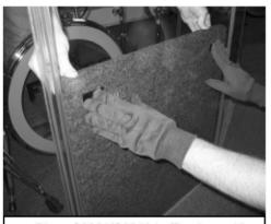
**8.** Place S2224/S2216 baffles in position on shields. Have assistant apply opposing pressure from opposite side then press baffle corners to secure Velcro to shield.
