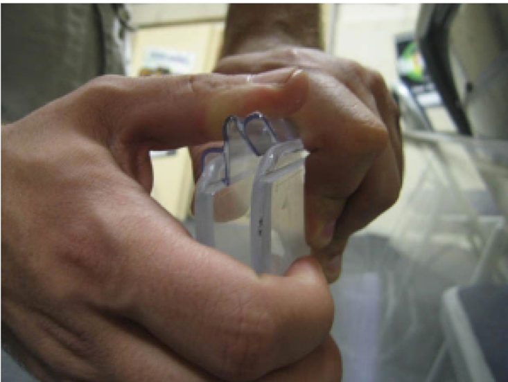
5. Bend hinge over onto adjoining panel and snap into groove. Attached completely to entire length of adjoining panel.
