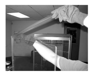
To install H-Channel: Outside edge of H-Channel should line up with outside edge of shield below.
