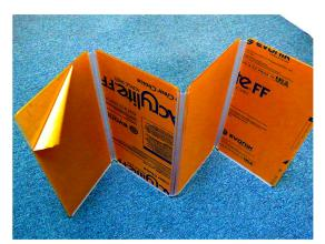
1. Stand acrylic panels up in a zigzag formation. Peel off paper masking. Note: this product is NOT returnable once paper masking is removed.
