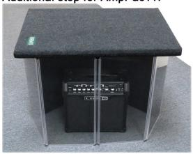
5. Place larger S2233 SORBER baffle on top so the front rests on the acrylic panels and the back rests on the S2224 SORBER baffles. There should be a small gap in the back to allow for air circulation. Your AmpPac11 is now complete!
