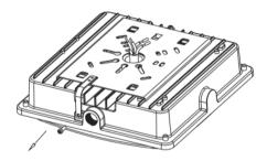
3. Screw the lamp and conduit pole together tightly.
