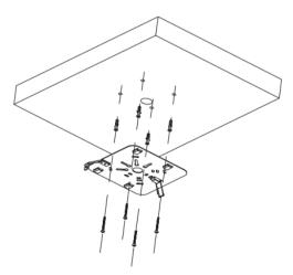
3. If you need to use the surface-mounted installation, a circle of glue is needed around the edge of the fixed plate.
