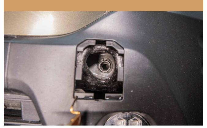
3 INSTALL NUT ONTO THE SUPPORT ROD
