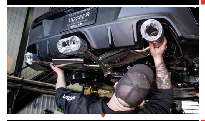
ATTACH THE EXHAUST HANGERS INTO THE RUBBER SUPPORTS
