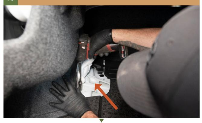
20 REMOVE STRUT AND REAR KNUCKLE BOLTS
