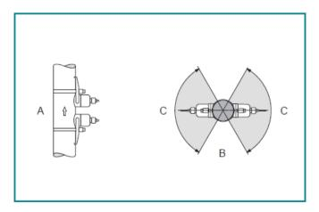
A is for upright pipeline, please notice the water direction is from the bottom to top.
