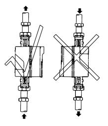
> For "U" type installation, the water meter should be in the lowest position to avoid air gathering in the pipe, causing meter inaccuracy.
