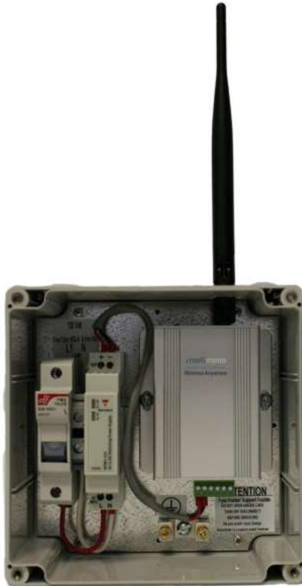
Integrated with a 2.4G RF modem and MCU, the i-meter®RS485 Wireless Radio module is designed to support low-cost and lower power wireless sensor networks. The radio module is enclosed in a polycarbonate enclosure with a hard-wired 120Volts power supply and a single-pole fuse holder.
