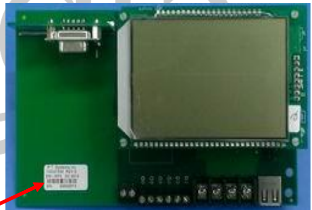
Examples of the Meter Serial Number Label Location on the PCB
