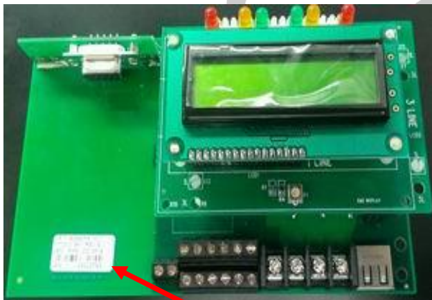
Examples of the Meter Serial Number Label Location on the PCB
