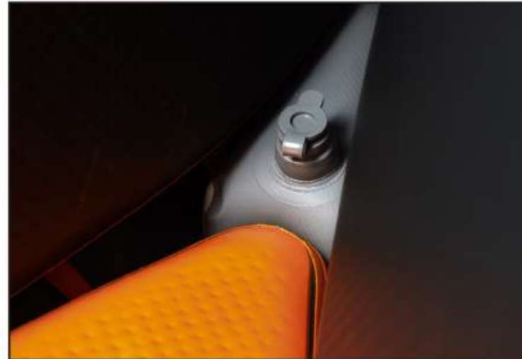
Inflatable keel design under bow and stern for remarkable tracking performance and efficient strokes
