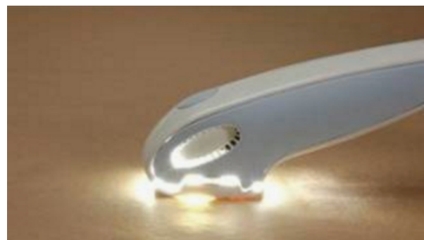
Figure 2. Silk’n device can only be fired upon complete contact of device tip with skin.
