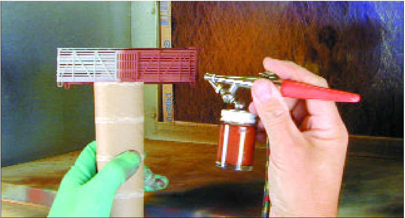
An airbrush is the paint applicator of choice for styrene models. Note the paper towel tube in use as a painting fixture, and the disposable plastic glove on the hand holding the model.
