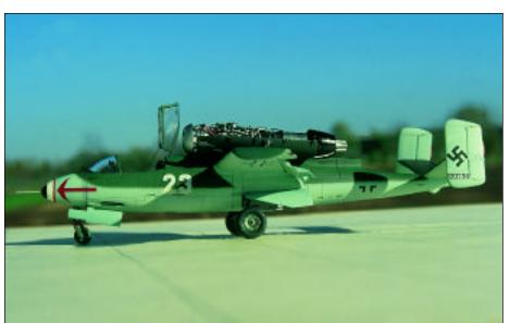
Bob Steinbrunn uses styrene extensively for both aircraft and ship models. His 1/48 scale Trimaster kit of the Heinkel He 162 Volksjager has been extensively modified and detailed with parts made from Evergreen sheet, strip, and rod.
