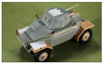
This diminutive 1/35 scale vehicle started as a Commanders kit of the World War II Hungarian Csaba armored car. Armor modeler Joe Morgan scratchbuilt the turret hatch, toolboxes on the rear fenders, and the antenna mounts from Evergreen styrene. The yet-to-be-painted model shows off his modifications.
