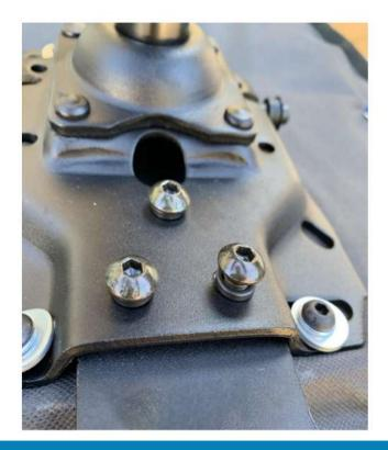
Tighten each bolt by hand a little bit at a time. It is important to rotate between all three bolts so that the pressure is evenly distributed.
