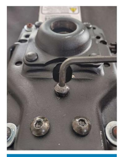
Complete the tightening process using the hex key
