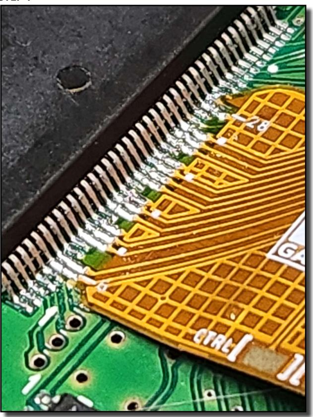
Solder the RCP flex cable starting at Pin 6 (as shown above).
