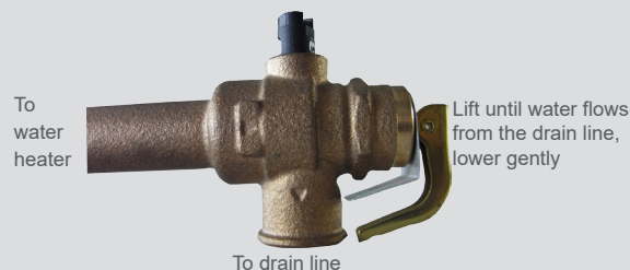
How to operate the easing gear
