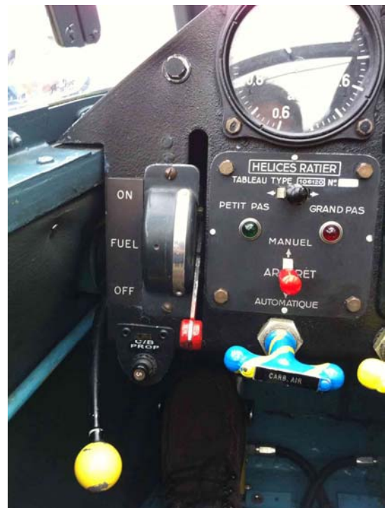
Propellor Control Subpanel (PCS)
