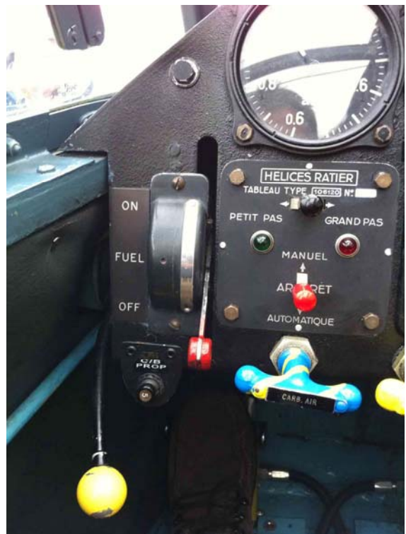
Propellor Control Subpanel (PCS)
