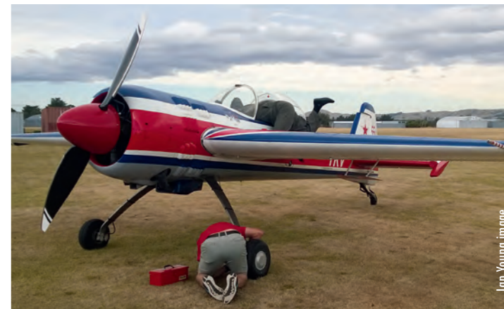
Bottoms up. Grant Benns helping Steve Geard bleed the brakes on his Yak-55.
