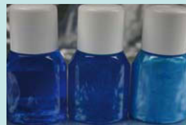
Figure 9. Examples for the effect of interference and silverwhite pigments in personal care products (from left to right): Gel with blue dye; gel with blue dye and 0.05 percent Ronastar® Green Sparks; gel with blue dye and 0.3 percent Timiron® Synwhite 40.
