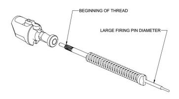
**CAUTION!** Carefully guide the firing pin into the shroud bore while compressing the spring. There is a precise fit inner diameter in the shroud that may catch on the beginning of the firing pin thread (shown below). Avoid applying excessive axial or bending force on the firing pin while compressing the spring.
