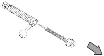
• Remove the firing pin assembly from the bolt.
