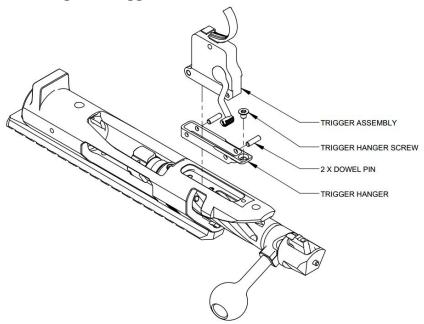
To install a Remington 700-compatible trigger:
