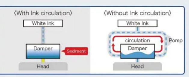
MCT Version2 (Mimaki Circulation Technology Version2) Circulation through out ink route including damper\*, supports stable white ink ejection for reducing frequent nozzle cleaning and ink waste.
