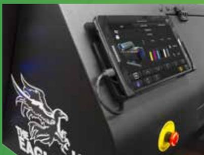
The printers remote management via tablet allows you to get an overview of the printer status and be able to perform routine management tasks without the need to physically visit the printer.
