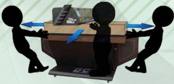
This innovative design allow to have three sides completely open that can be used to load and unload the table. You can remove printed objects and reload the table while the machine is still printing and it's particularly useful when you need to load bulky objects on the print table.
