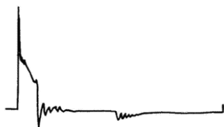
Secondary circuit resistance is too large
