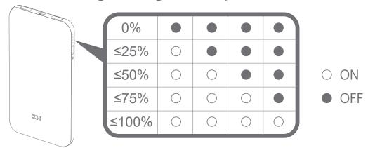
NOTE: The charge level check button is not a typical ON/OFF switch. A single press will wake up the device from sleep, but will not turn it off if already on. By design, the device (including the lights) will turn off automatically within 30 seconds after it has gone idle.
