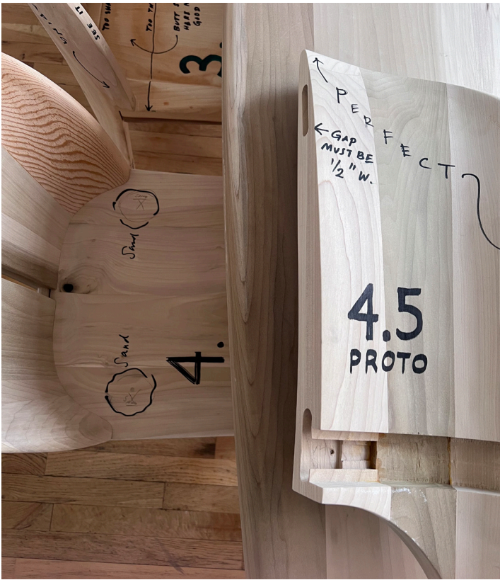
PROTOTYPE OF THE OVO CHAIR WITH DESIGN AND CONSTRUCTION NOTES.
