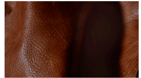
COMPOSITION COW HIDE CODE SW COW SB03 COLOR SADDLE BROWN WEIGHT 3OZ FINISH WAXED AVG. HIDE SIZE 20SF
