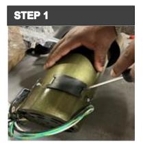
Remove the motor brush cap with a flat head screwdriver.
