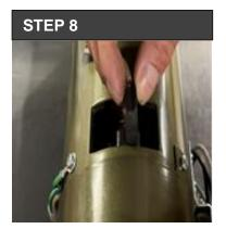
Insert motor brush into brush holder. With twist tie still attached to motor brush spring, insert spring back into the holder. Once secured, remove the twist tie.
