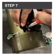
Using needle nose pliers, reattach the motor brush wire to the terminal that you originally removed it from. (See Step 3 for reference)
