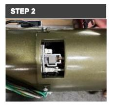
The motor brush spring and motor brushes will be exposed.
