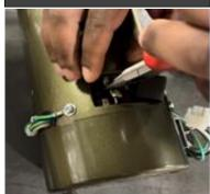
Using needle nose pliers, remove the motor brush wires from the connector.
