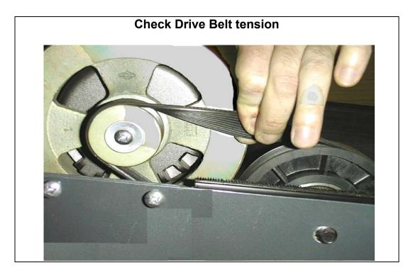
Drive Belts are pretension before the treadmill leaves the factory. Adjustments are ONLY necessary when Drive Belt is slipping during use. If the belt needs to be adjusted use a 7/16" socket and turn the bolt underneath the motor pan attached to the hook screw.
