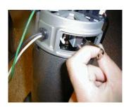
Press down on the metal spring, slide the motor brush holder and take the clip out.
