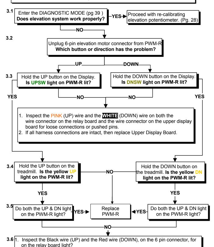
2. If all harness connections are intact then replace the Elevation Motor.
