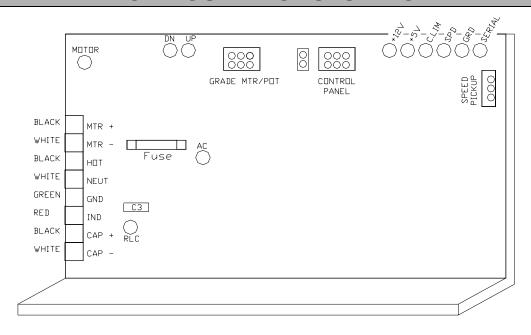
The SCR lower board is designed with diagnostic LED lights. The LED's are color coded according to their specific function. Green indicates a properly operating treadmill; the green lights should always be ON when power is supplied to the treadmill. Yellow indicates a treadmill function. Red indicates a treadmill malfunction. Here is a list of each LED and what it signifies:
