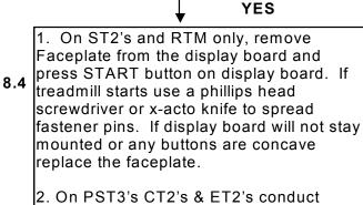
Membrane bypass test (See page 41) If treadmill starts replace Membrane Panel. If not replace the upper display board.
