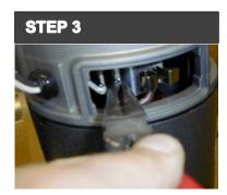
Using needle nose pliers, remove the motor brush wires from the connector.
