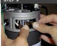
Insert the motor brush cover back onto the drive motor. Repeat all steps on the opposite side. Once both sides are completed, plug the treadmill back into the wall outlet.
