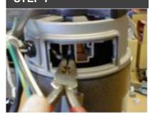
Using needle nose pliers, reattach the motor brush wire to the terminal that you originally removed it from. (See step 3 for reference)
